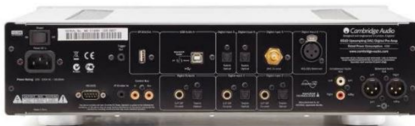
The 851D accepts PCM data up to 192kHz on all inputs except USB.
