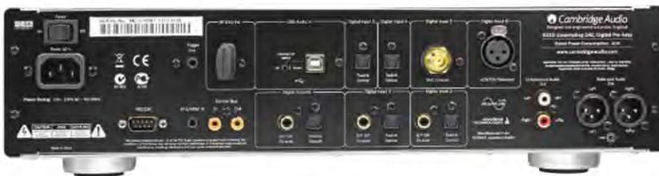
Practically any digital source can be fed into the 851D. There are no fewer than six digital audio inputs plus a pair of USB ports for computer DAC and Bluetooth use. The analogue output is available in unbalanced (phono) and balanced (XLR) form. The 851D also makes provision for custom installation (RS232, remote in, 12V DC trigger out and Cambridge's control bus).
