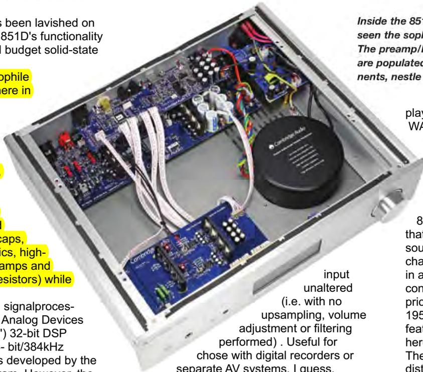
Inside the 851D. At the bottom left can be seen the sophisticated headphone amplifier. The preamp/DAC and terminal boards, which are populated with decent-quality components, nestle around the rear panel.
